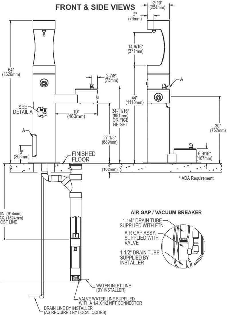
**SANITARY FREEZE-RESISTANT VALVE GROUND INSTALL DETAIL**
